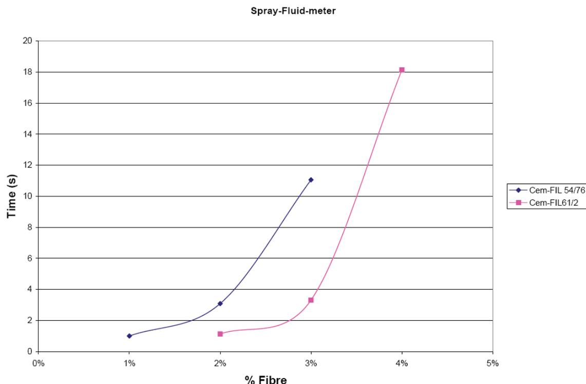
Figure 16: Fluid-meter. Spray product viscosity vs percentage fibre content
