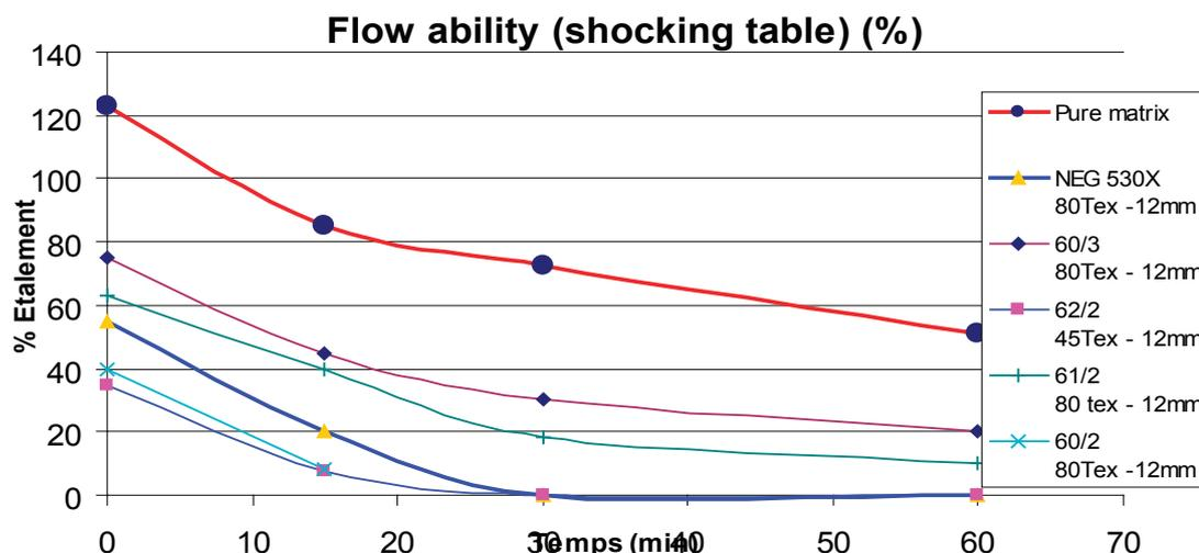
Figure 12: Viscosity = f (time) for different strands (w/c = 0.34; fibres = 3.5%)
