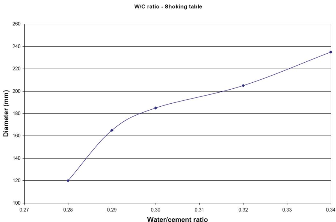
Figure 9: Shaker table. Paste viscosity vs w/c ratio
