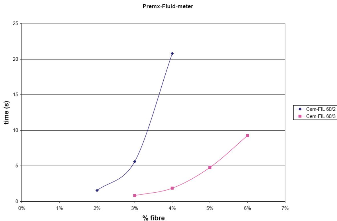
Figure 15: Fluid-meter. Premix product viscosity vs percentage fibre content
