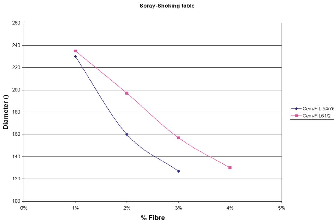
Figure 11: Shaker table. Spray product's viscosity vs percentage of fibre content
